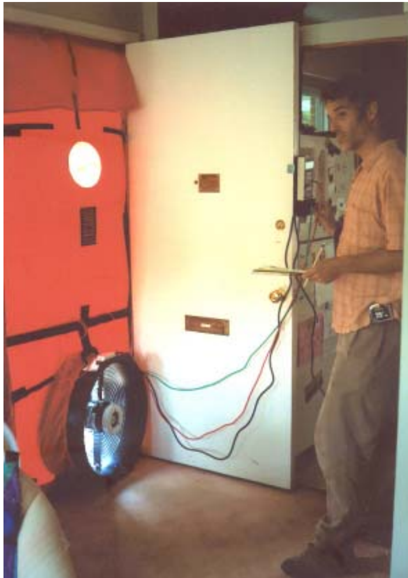
Walder uses a "blower door" to test for air infiltration.
